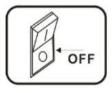
1. Turn off the power to the luminaire before removing the lamp.
