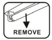
3b. Then, remove the lamp from lampholder.
