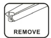
2. Remove the diffuser lens/ cover (if applicable).
